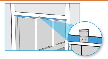
Using the spacer as your placement guide, position the open ends of each glide base adjacent to each side of the installed spacer. Both glide bases need to align on the sides and be level with the bottom of the spacer as illustrated. Use three 1" stainless steel Tek screws from Door Kits to attach each glide base. Continue with Step 12 in the Original Sliding Screen Door Instructions for attaching each glide base.
